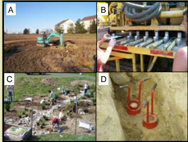
Figure 1. Examples of common practices consulting soil scientists are undertaking in Pennsylvania: (A) Site investigations; (B) Split spoon sampling analysis; (C) Rain garden installation; (D) Double ring infiltrometer.
